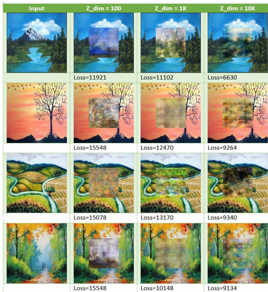
Figure 9: Z Vector Dimension Tuning for GoogleImages DCGAN Inpainting
