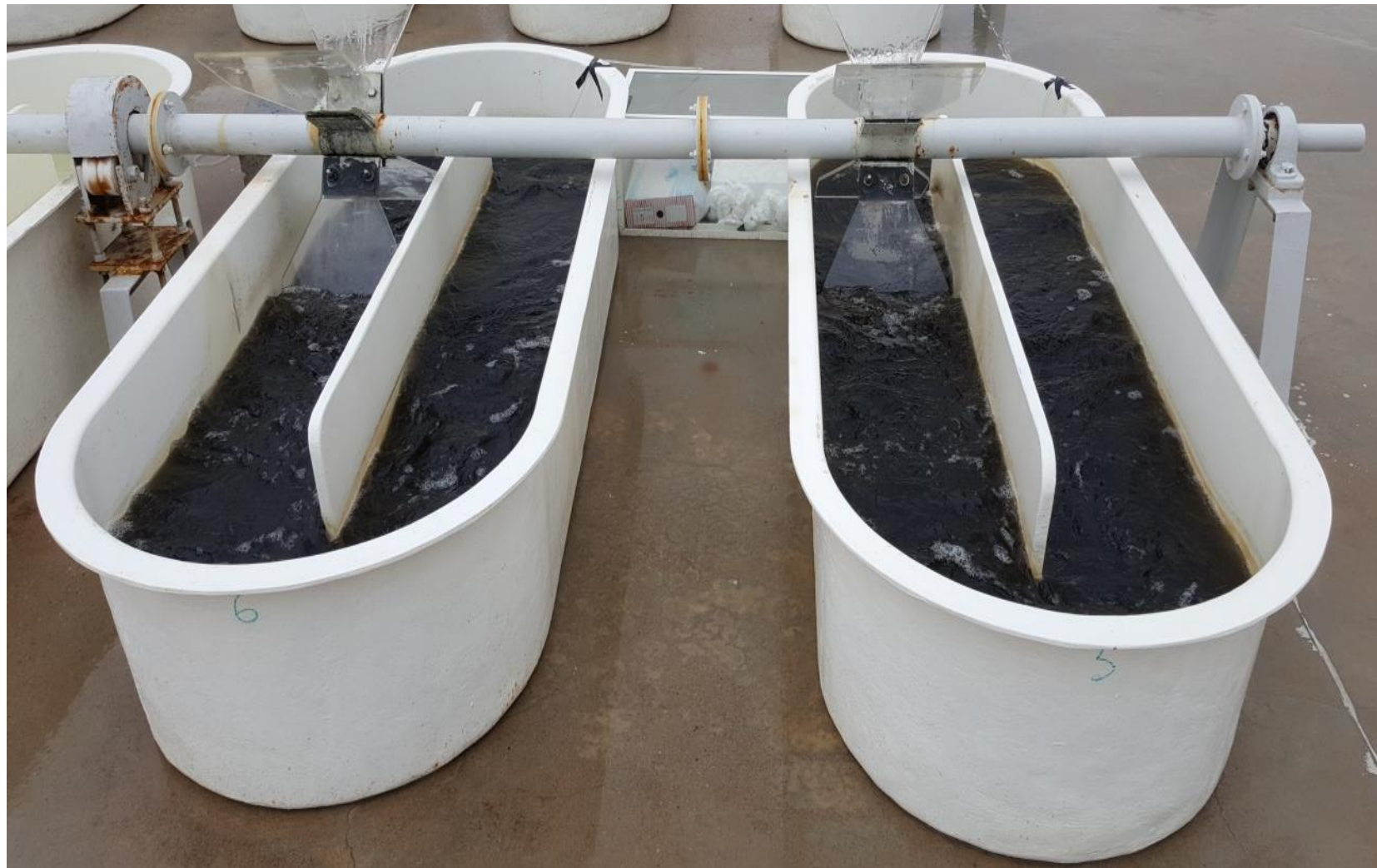
Outdoor continuous cultivation of Chroococidiopsis sp. in 200 L raceway tanks
