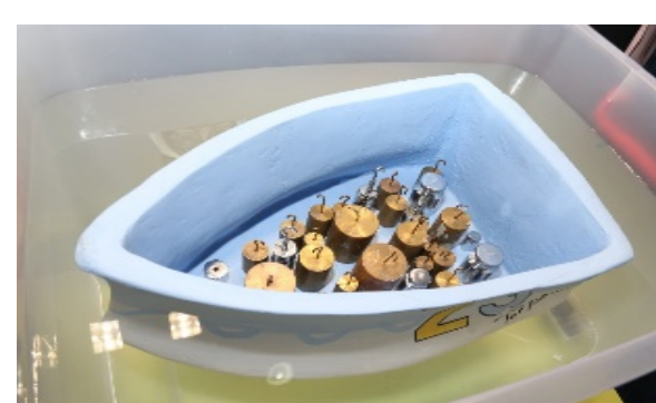
Figure 1 Concrete boat floating and carrying load
