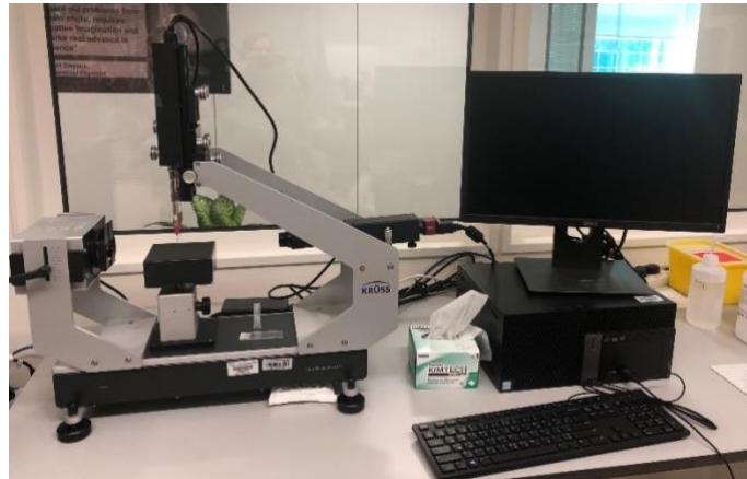
Figure 28. KRUSS Drop Shape Analyzer DSA25 equipped with a camera and photo analysis system.
