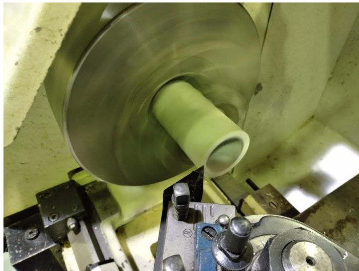
Figure 17. The sample being faced using a turning machine
