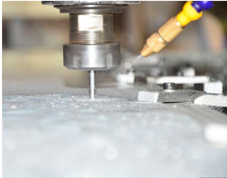
Figure 24. CNC machine used for machining foam cores
