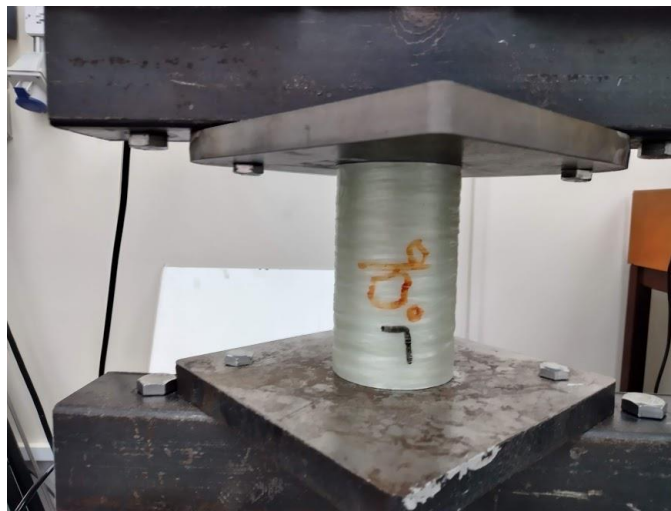
Figure 20. Sample positioned between compressive plates before the test
