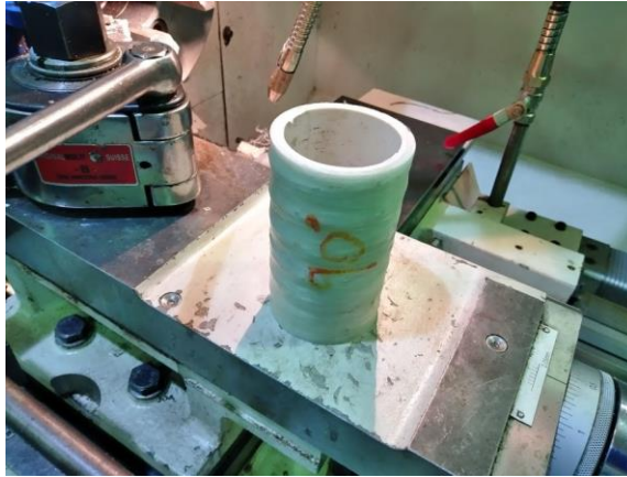
Figure 19. Completed sample with an uneven surface
