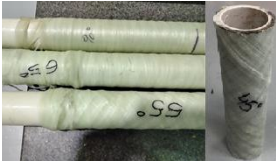
Figure 15. Glass fiber/epoxy overwrapped PVC pipes before cutting
