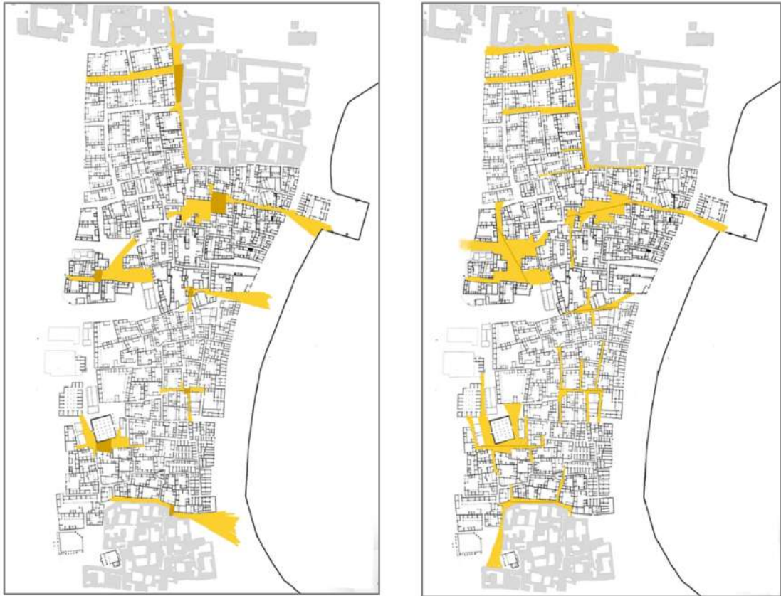
Figure 57: Representation of a visual field (in yellow) from a line, and convex space in the plan of Souq Al Wakrah, State of Qatar (Source: Author).
