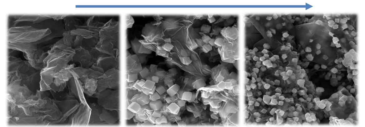
**SEM** showed the formation of Ge-cubes after ball-milling treatment with average size of 0.8 to 1.2  $\mu m$ . Increased Ge mass loading lead to greater surface distribution of Ge cubes above the r-GO sheets.
