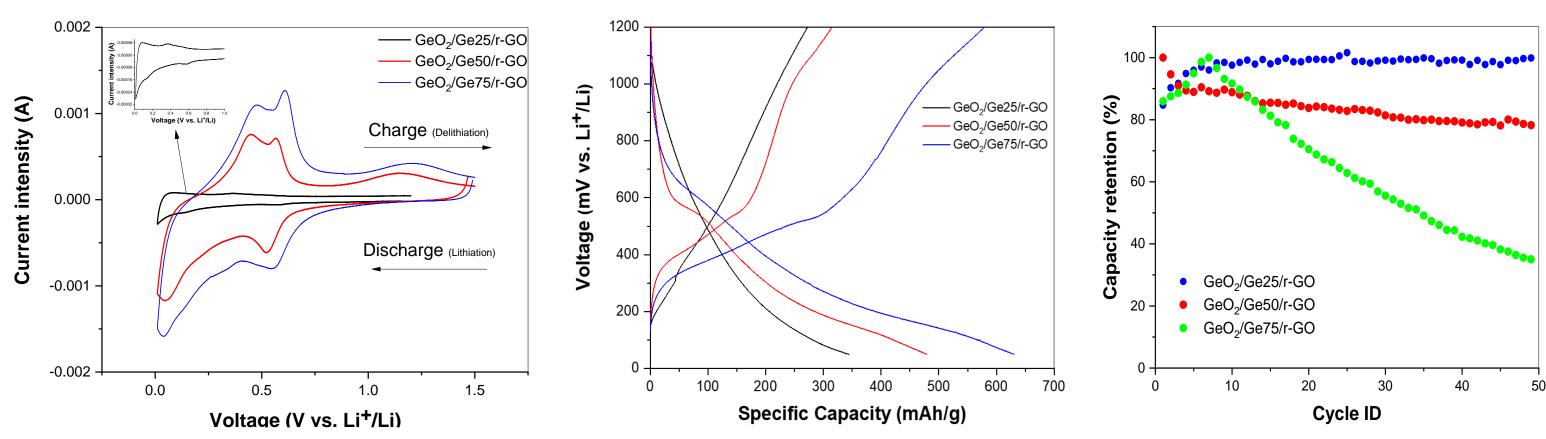
Three wt.% compared in CV and GCD tests. CV showed peak development and transitioning with increased wt.%. GCD tests show increased initial charge and discharge values with decreased cycling retention with increased wt.%.
