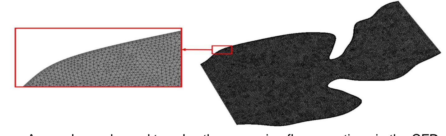
A sample mesh used to solve the governing flow equations in the CFD analysis. The mesh density is increased near the walls in order to improve the solution accuracy.
