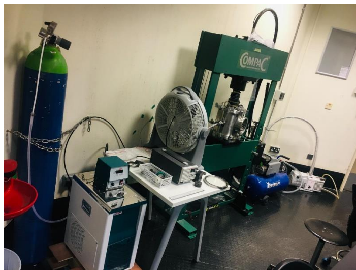
Figure 8: The vacuum hot press system used to compact the processed powders.
