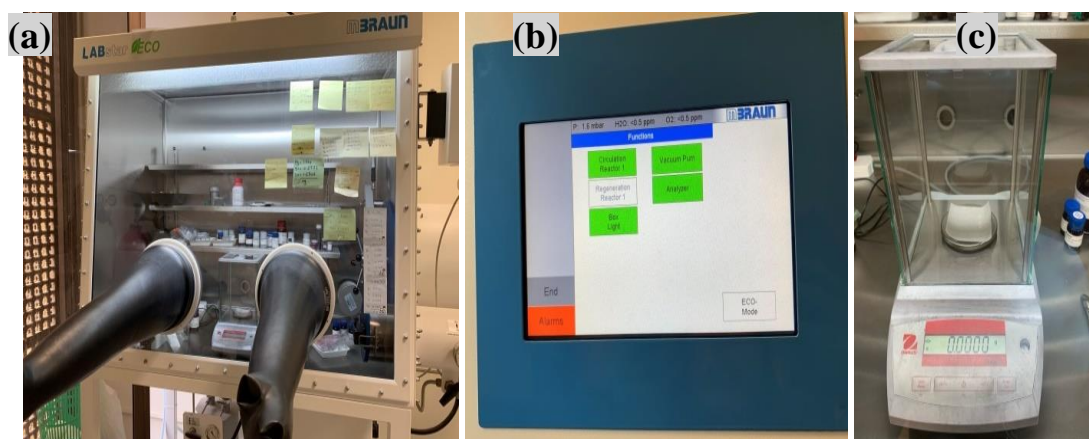
Figure 7: The mBRAUN-LABstar (a) Glovebox workstation and (b) its touch panel (c) along with Ohaus balance weighing equipment.
