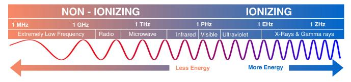
FIGURE 1. Ionizing and Non-ionizing radiation sources and there frequency bands.
