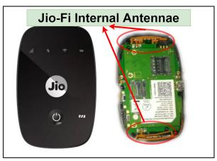
(b) Antennas in a portable Wi-Fi router
