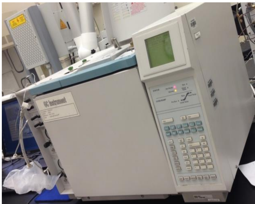
Figure 15: GC-MS system while testing the evolved gas from 1 st cut SPL samples after washing with deionized water
