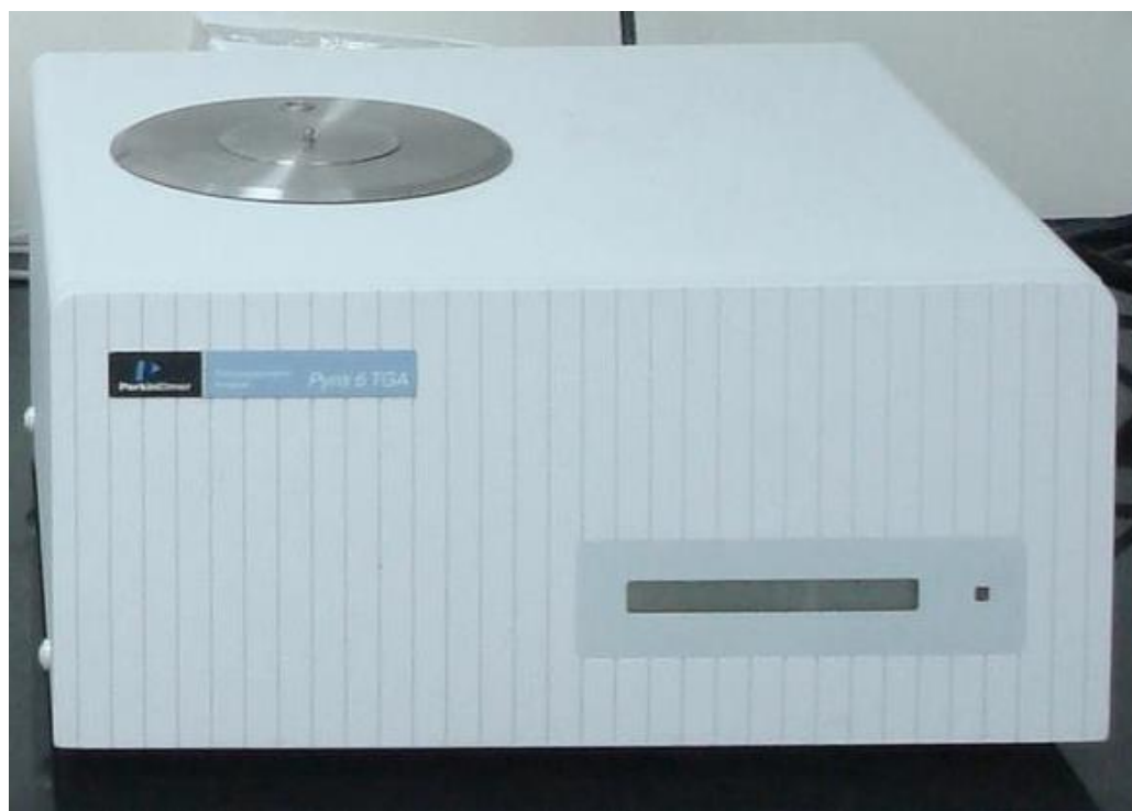
Figure 17: TGA instrument that was used to measure thermograms for different 1 st cut SPL samples
