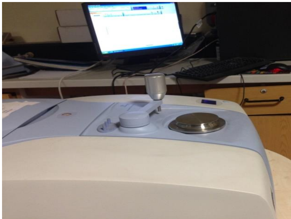
Figure 16: FTIR instrument that was used to qualitatively analyze the 1 st cut SPL samples.
