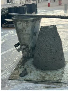
Fig. 3: Slump test for S0-P0
