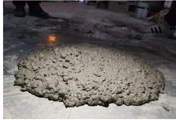
Fig. 4: Collapse slump for S33-P0.5
