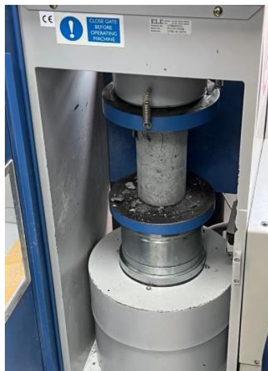
Fig. 5: Compression test set-up
