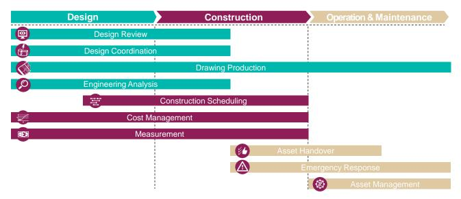
Fig. 4: Main Ashghal BIM Uses
