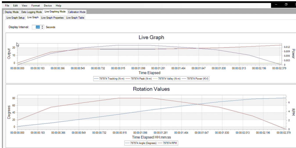
Figure 3B: Real-time data plot in Futek rotary sensor application
