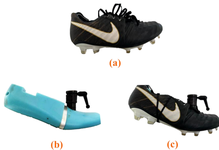
Figure 18. Fitted shoe on dummy shoe holder at 20° of plantar flexion
