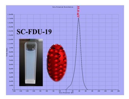
Figure S12. Zeta potential values ( $\zeta$ ) of the mesoporous TiO<sub>2</sub> single-crystals SC-FDU-19 dispersed in water as shown in inset, revealing that all the charges are positive.
