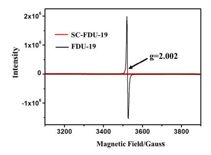
Figure S11. The electron paramagnetic resonance (EPR) spectra of the mesoporous  $TiO_2$  mesocrystals FUD-19 and mesoporous  $TiO_2$  single-crystals SC-FDU-19. The spectra are recorded at room temperature (25 °C).
