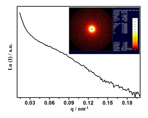
**Figure S22.** The small-angle X-ray scattering (SAXS) pattern of the as-made FDU-19. Inset is the corresponding 2D SAXS image of the as-made FDU-19.
