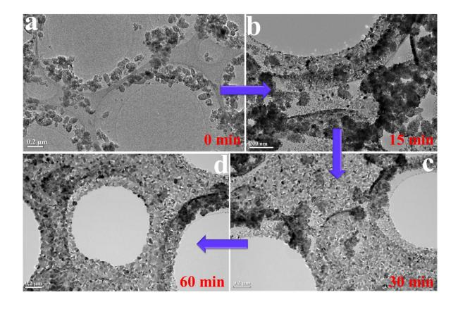
Figure S17. The *in-situ* TEM images of intermediates for NS-FDU-19 harvested at different intervals of time (a), 0 min, (b), 15 min, (c), 30 min and (d), 60 min. The *in-situ* TEM heating experiment was carried out at 400 °C in a high vacuum (~  $4.0 \times 10^{-5}$  Pa) on a grid with molybdenum supporting film using the EM-21130 Specimen Heating Holder.
