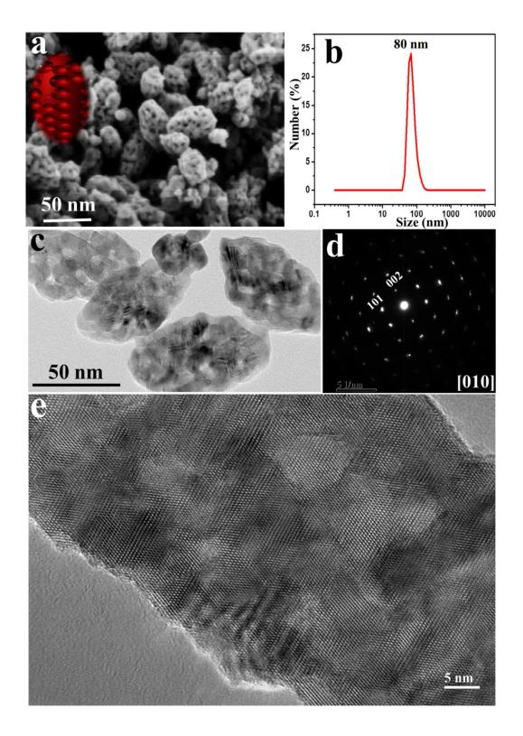
Figure S13. (a) The typical SEM image, (b) dynamic light scattering (DLS) spectrum, (c) TEM image of the mesoporous TiO<sub>2</sub> particles SC-FDU-19 with an average size of  $\sim 80$  nm; (d) SAED patterns, (e) HRTEM image of a single particle SC-FDU-19 with a size of  $\sim 80$  nm recorded along [010] axis.
