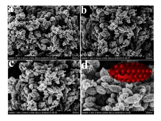
**Figure S8.** SEM images of the mesoporous  $TiO_2$  single-crystals SC-FDU-19 after the calcination in air at 400 °C for 2 h, showing that the annealing in air can drive a regular 3D *in-situ* fusion of the mesopore mesochannels of the mesocrystals FUD-19 into 3D open spherical mesopores. Inset (d) is the schematic illustration of the mesoporous TiO<sub>2</sub> single-crystals SC-FDU-19.
