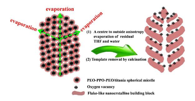
**Figure S21.** Schematic representation of the formation process of curving cylindrical channels within the olive-like mesoporous TiO<sub>2</sub> mesocrystals through the evaporation-driven oriented assembly process.
