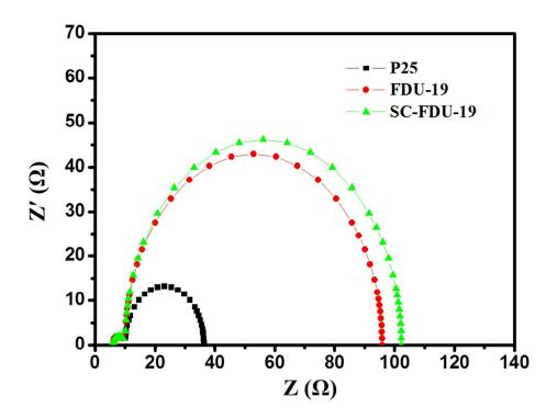
**Figure S24.** Nyquist plots of FDU-19, SC-FDU-19 and P25-based DSSCs (with the same photoanode film thickness of about 13  $\mu$ m) measured at -0.8 V forward bias in dark.
