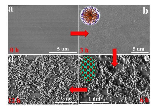
**Figure S2.** *Cryo*-SEM images of the samples harvested from THF/F127/H<sub>2</sub>O/HCl/HOAc/TBOT mixed acidic solution at different intervals of time (**a**), 0 h, (**b**), 3 h, (**c**), 6 h and (**d**), 12 h.
