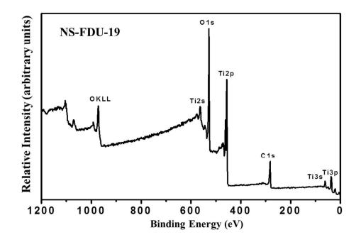
Figure S15. The XPS spectrum of the single-crystal TiO<sub>2</sub> nanosheets NS-FDU-19.
