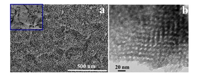
Figure S4. (a) SEM and (b) TEM image of the mesoporous  $TiO_2$  bulks obtained with the aid of swelling 1,3,5-trimethylbenzene (TMB) molecules. Inset (a) is the overall morphology of the mesoporous  $TiO_2$  bulks.
