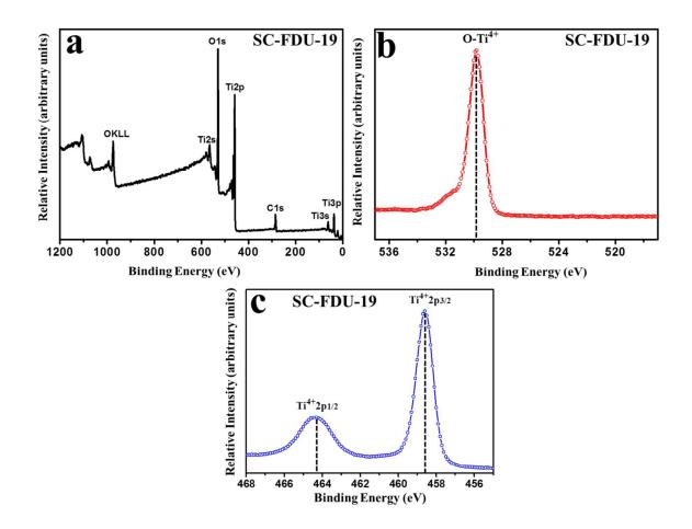
**Figure S10. (a)** The X-ray photoelectron spectra (XPS) of the mesoporous TiO<sub>2</sub> single-crystals SC-FDU-19, showing two characteristic peaks of Ti and O; (b) O1s XPS core-level spectra for SC-FDU-19. (c) Ti 2p XPS core-level spectra for SC-FDU-19.
