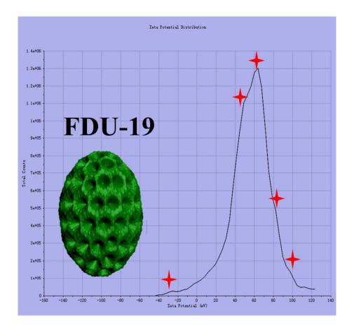
**Figure. S7.** Zeta potential value ( $\zeta$ ) of the mesoporous TiO<sub>2</sub> mesocrystals FDU-19 dispersed in water, showing the existence of mainly positive charges and a few negative charges.
