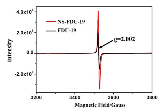
**Figure S16.** The electron paramagnetic resonance (EPR) spectra of the mesoporous  $TiO_2$  mesocrystals FUD-19 and mesoporous  $TiO_2$  single-crystals NS-FDU-19. The spectra are recorded at room temperature (25 °C).
