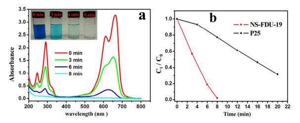
**Figure S25.** Photocatalytic decomposition of methylene blue dye  $(1.0 \times 10^{-4} \text{ mol } \text{L}^{-1}, 50 \text{ ml})$  over the TiO<sub>2</sub> single-crystal nanosheets NS-FDU-19 and Degussa TiO<sub>2</sub> P25. (**a**) UV-vis absorption spectra and corresponding color changes of the methylene blue solution (inset). (**b**) C<sub>t</sub>/C<sub>0</sub> vs time curves of methylene blue photodegration over NS-FDU-19 and Degussa P25.
