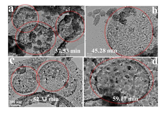
**Figure S20.** (a-d) The *in-situ* TEM images of the  $TiO_2$  nanosheets NS-FDU-19 harvested at different intervals of time, showing that the freshly-formed SN-FDU-19 nanosheets are free-standing on the TEM grids with molybdenum supporting film in a spherical symmetry.
