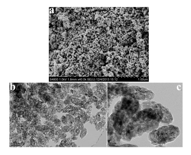
Figure S14. SEM (a) and TEM (b, c) images of the mesoporous  $TiO_2$  single-crystal particles SC-FDU-19 with an average size of ~ 100 nm.
