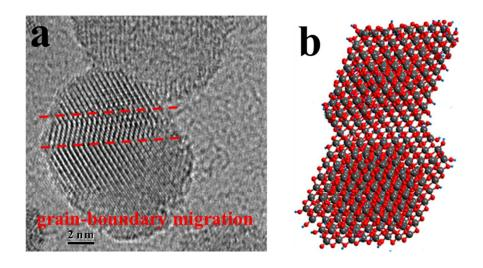
**Figure S19. (a)** The *in-situ* HRTEM image of an intermediate during the formation of NS-FDU-19 nanosheets harvested at 25.17 min. **(b)** The corresponding crystallographic simulation, showing that the monolayer-reconstruction undergoes an atom-by-atom reorientation *via* grain-boundary migration.
