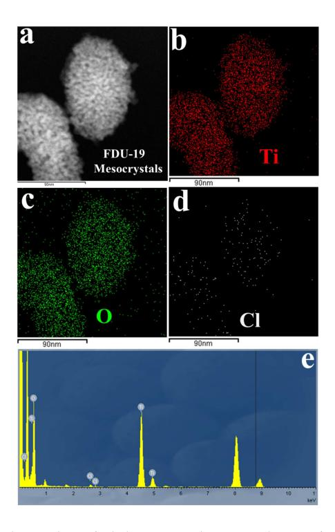
**Figure S6**. (a), The STEM image of a single mesoporous  $TiO_2$  mesocrystal FDU-19 after calcination in  $N_2$  at 350 °C for 2 h; (b-e), EDX elemental maps of Ti, O and Cl, respectively, for a single mesocrystal FDU-19, showing a small amount of Cl<sup>-</sup> ions adsorption on the surface.
