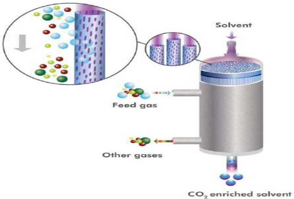
Figure 1.3. Gas absorption membrane principle using hollow fiber membrane 25 .
