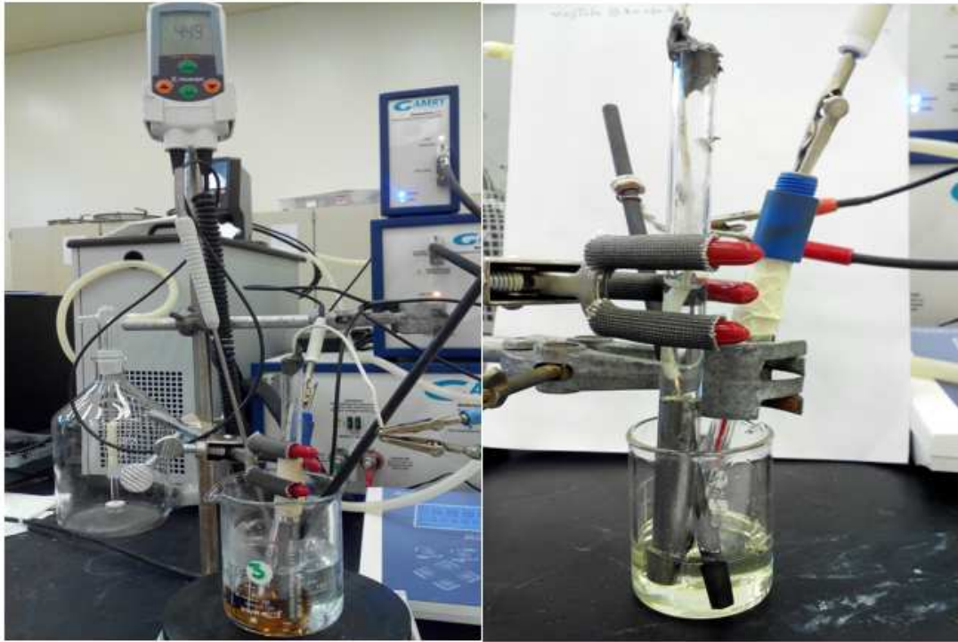
Figure 3.9. Set up of corrosion test.
