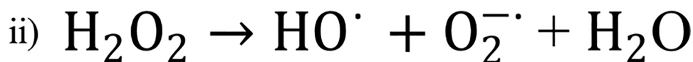
Figure 2. hydrogen peroxide decomposition reaction and generation of hydroxyl radical and a superoxide anion.
