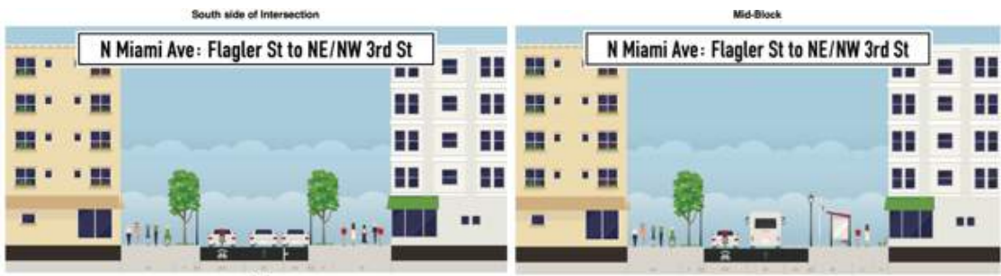
Figure 8. Proposed Cross-Section of the Selected Corridor Using 'Complete Streets' Principles (Source: Miami-Dade, 2014)
