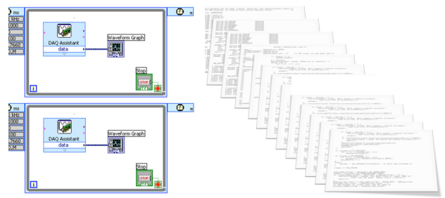
Figure 5. Comparing ‘G’-based with Textual-based code for two parallel DAQ timed-loops
