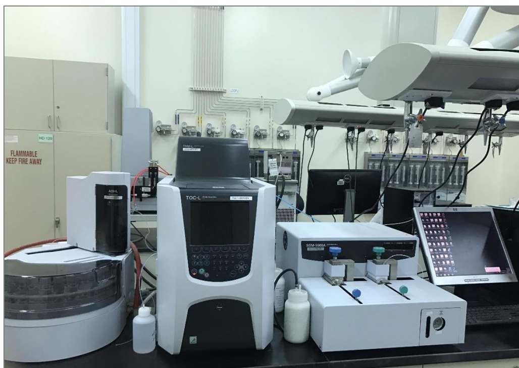
Figure 3. 11: Total Organic Carbon Analyzer TOC-L (Shimadzu, Japan)
