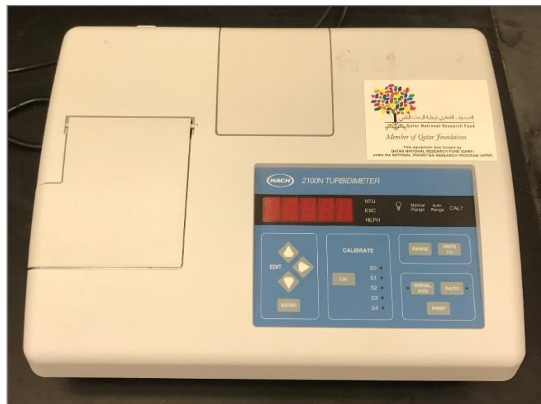
Figure 3. 12: Hach 2100N bench top turbidity meter
