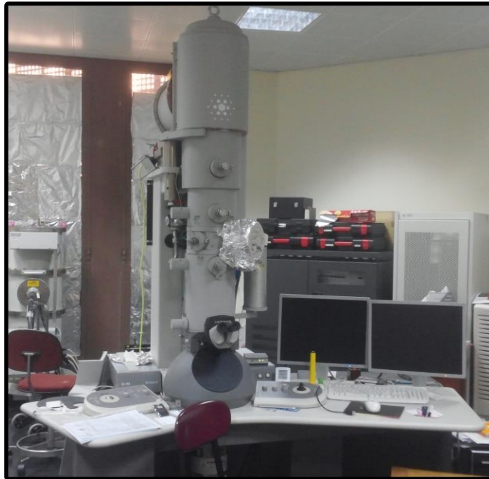
Figure 3-8: Transmission electron microscope setup.
