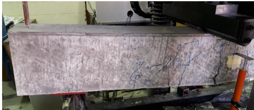
Figure 43. Beam A8 (Compression flexural failure)
