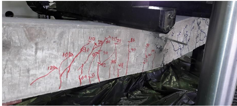
Figure 39. Beam A4 (Compression flexural failure)
