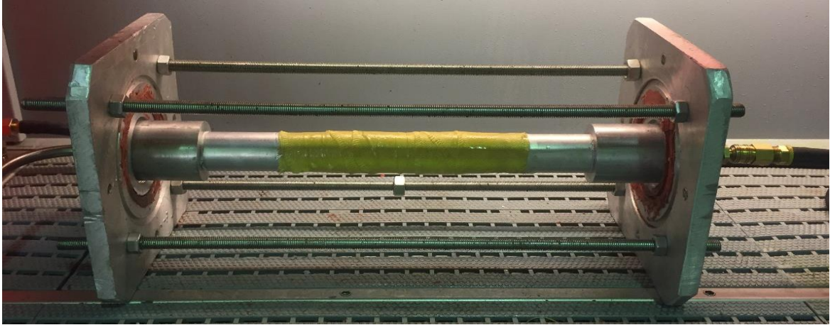
Figure 3.12: Fixation for radial internal pressure test.
