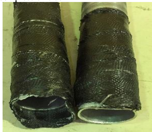
(d): 0^\circ/90^\circ CFRP joining failure in compression side
