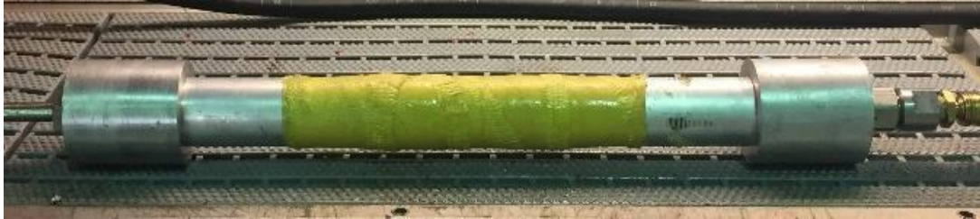
Figure 4.27: Aluminum pipe joined with KFRP joining under combined axial and radial internal pressure test.
