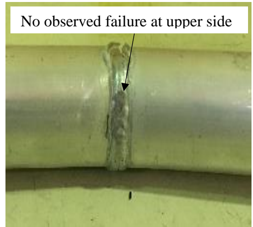
(f): Normal faced welded pipe fracture in upper side
