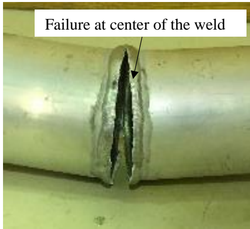
(e): Normal faced welded pipe fracture in lower side
