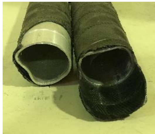
(b): \pm 45^\circ CFRP joining failure in compression side
