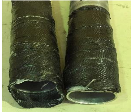
(d): CFRP failure in compression side
