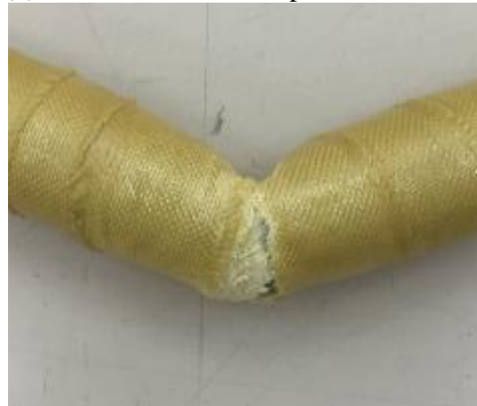
(f): KFRP failure in compression side
