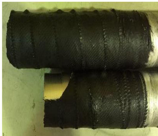
(a): \pm 45^\circ CFRP joining failure in tension side
