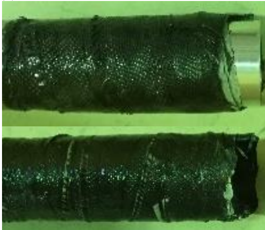
(c): CFRP failure in tension side
