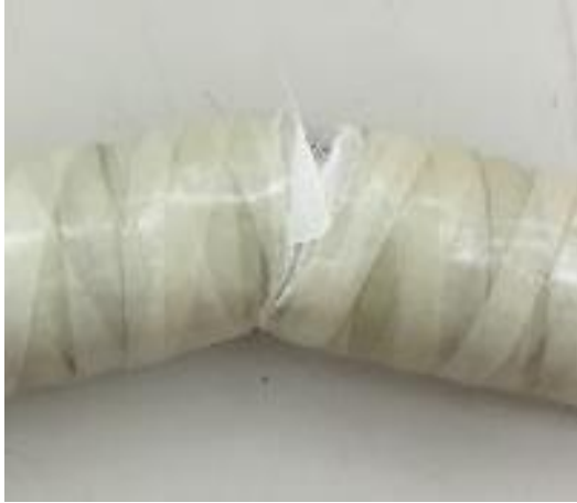
(a): GFRP failure in tension side
