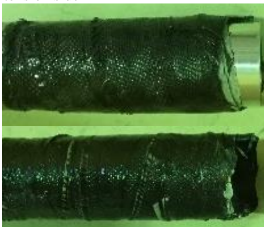
(c): 0^\circ/90^\circ CFRP joining failure in tension side
