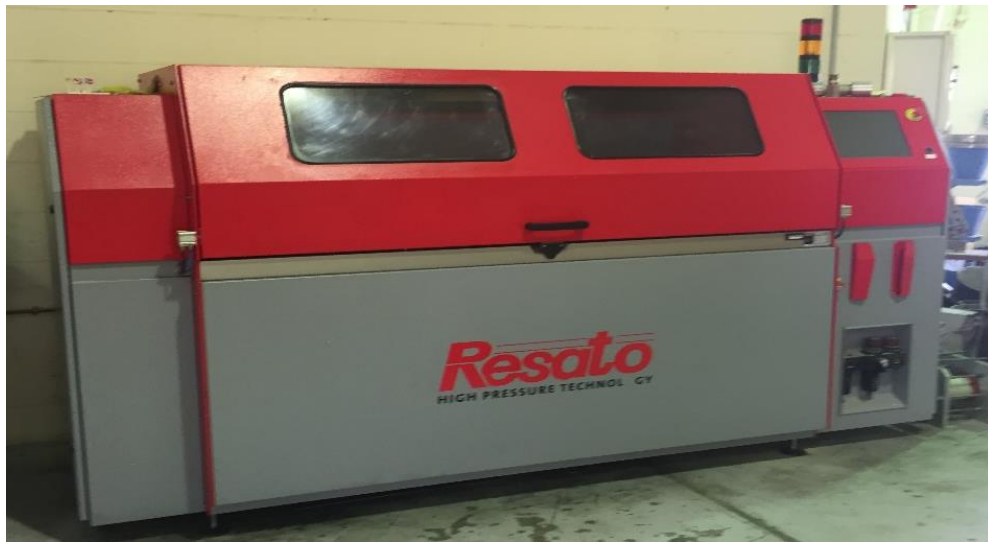
Figure 3.9: Resato high-pressure testing machine.
