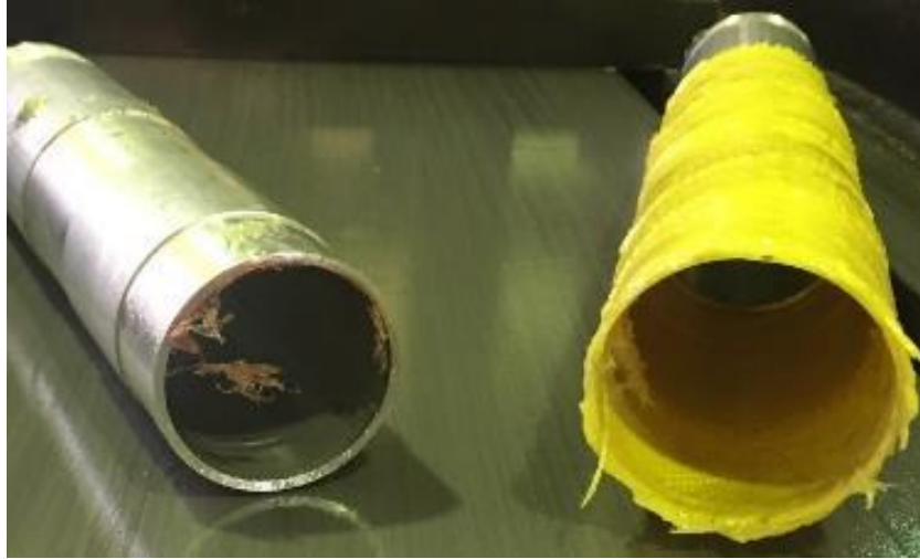
Figure 4.29: Splitting of the joint from the pipe.
