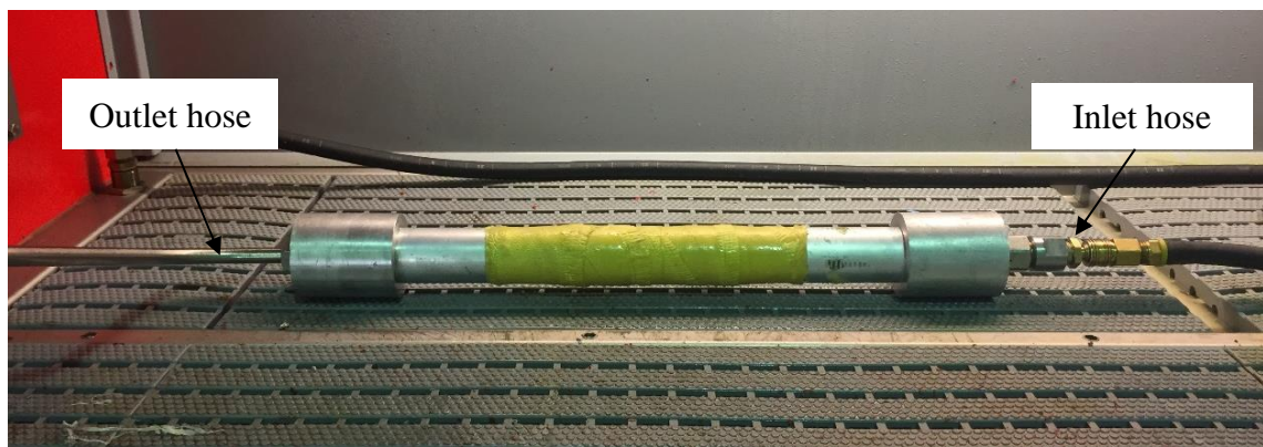
Figure 3.11: Pipe after fixation with inlet and outlet hoses for combined axial and radial internal pressure test.
