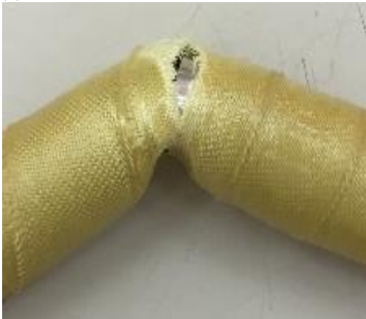
(e): KFRP failure in tension side
