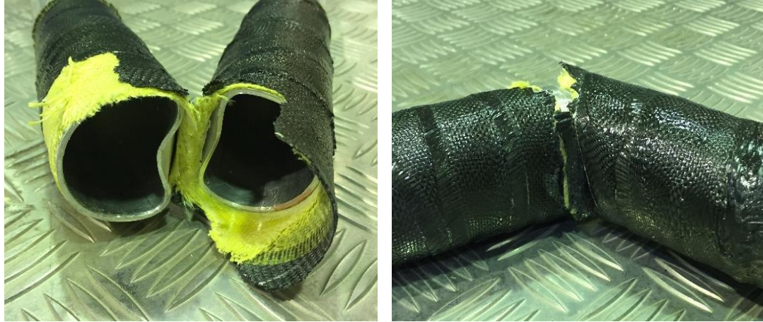
(a): KFRP/CFRP joined pipe failure in tension side
