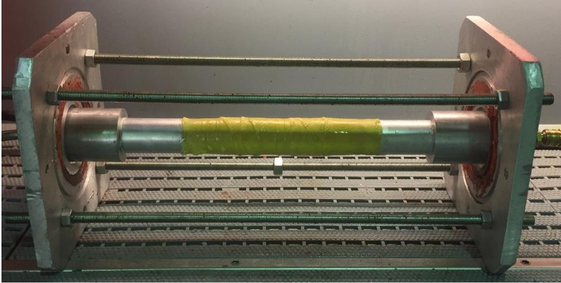
Figure 4.30: Fixation for radial internal pressure test.
