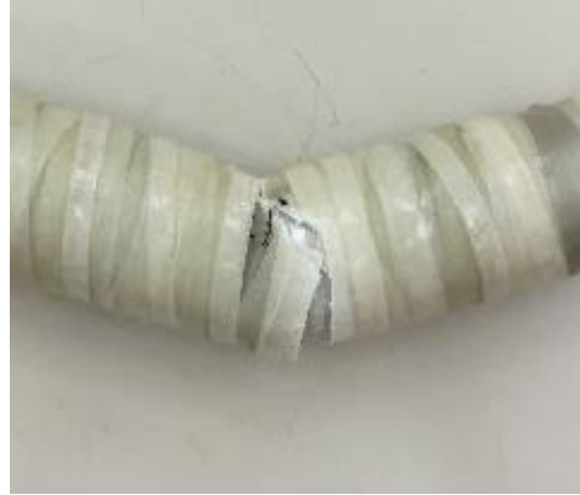
(b): GFRP failure in compression side
