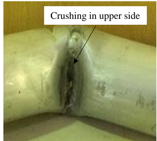
(d): V-welded pipe crushed in upper side
