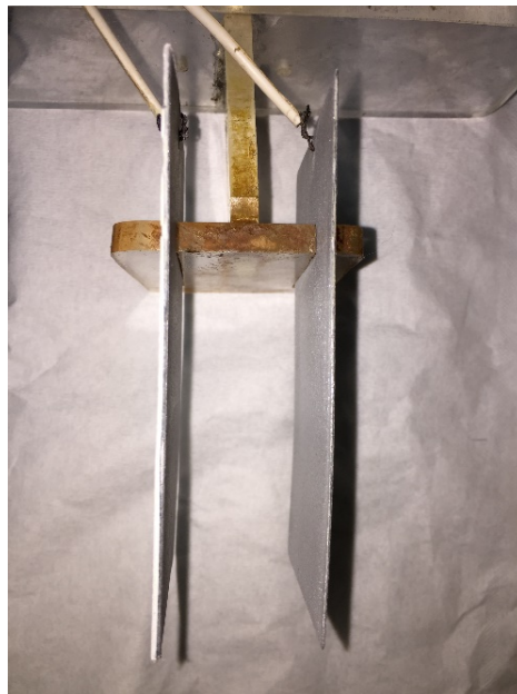
Figure 7: The Aluminum Plates Used as Anode and Cathode on PVC Mount.
