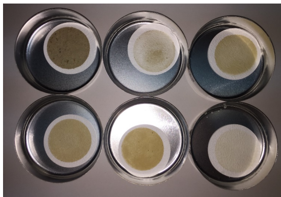
Figure 15: Drying Filter Paper Used for Calculating Total Suspended Solids.
