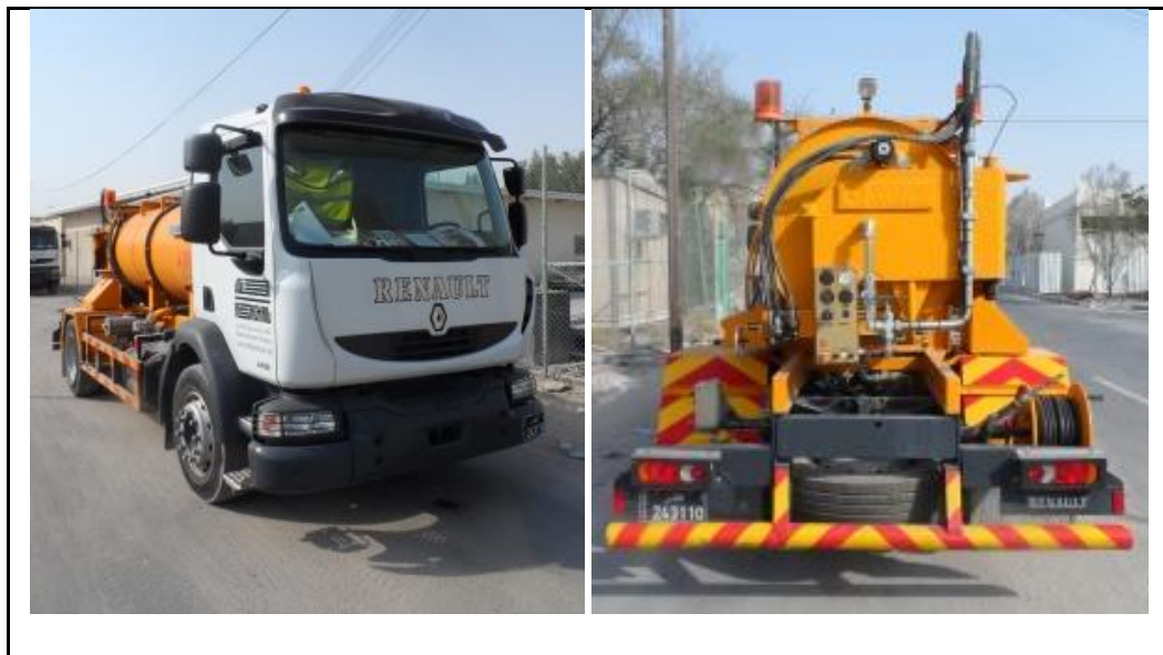
Figure 8. Jetting Tanker (Jetter)
