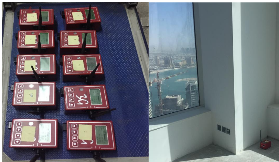
Figure 29: wireless Sensors Setup – TROMINO-
