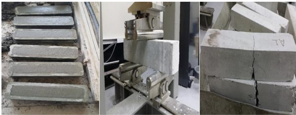
Figure 10. Concrete Prism Samples Before, During and After Testing
