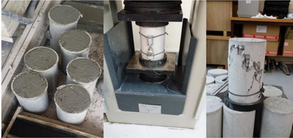
Figure 8. Concrete Cylindrical Samples Before, During and After Testing
