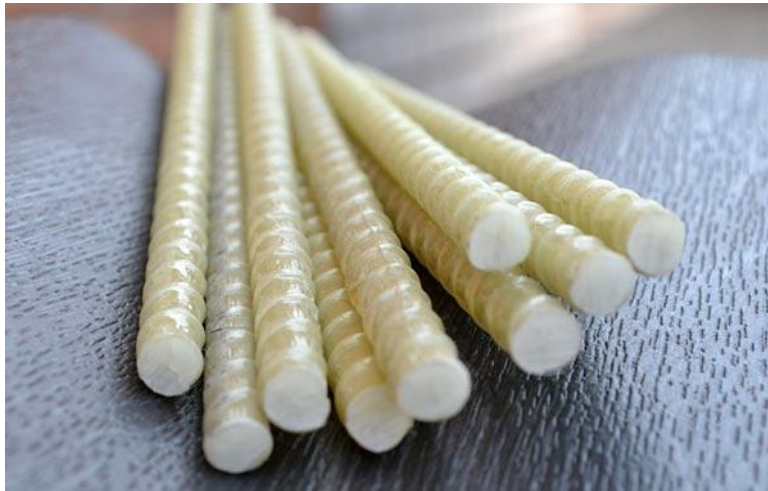
Figure 4. GFRP Reinforcing Bars
