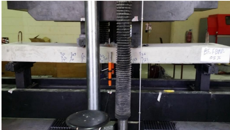
Figure 18. One-Way Concrete Slab during Test
