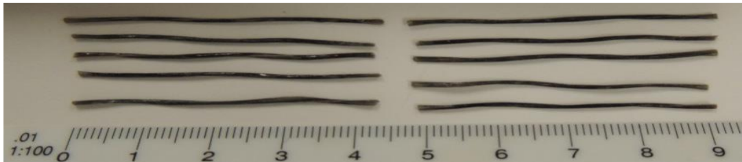
Figure 2. Length of Basalt Macro-Fibers
