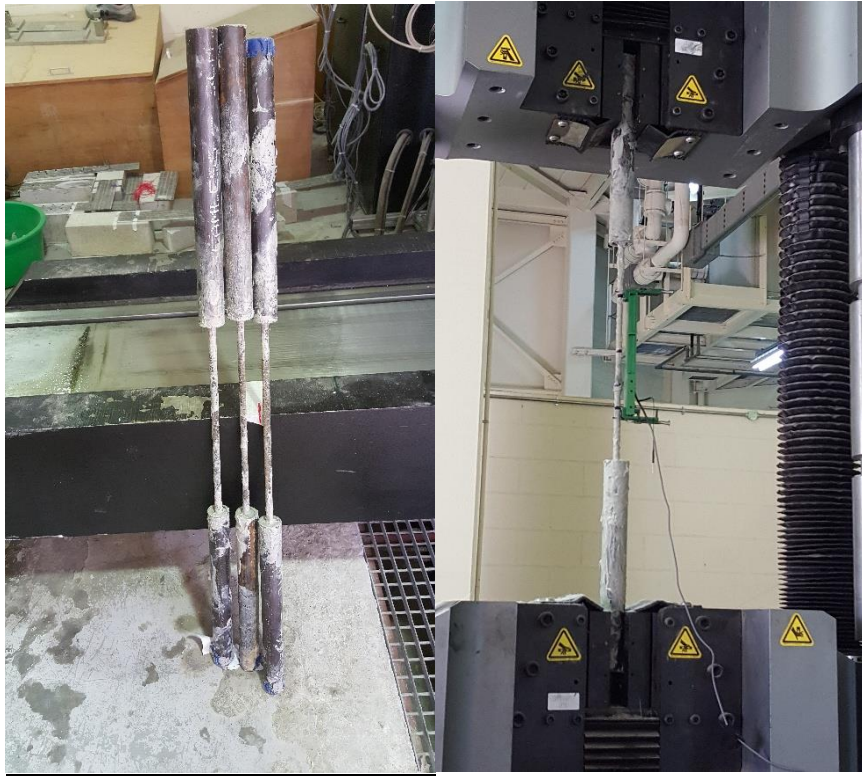
Figure 6. FRP Reinforcing Bars under Tensile Strength Test
