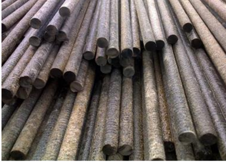
Figure 3. BFRP Reinforcing Bars
