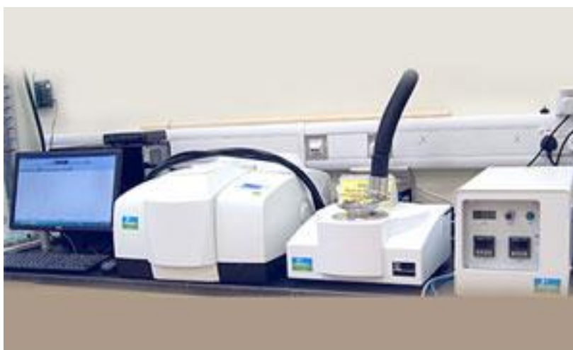
Figure 12: TGA FTIR set up (FT-IR Spectrometer Frontier/ TGA 4000 – Perkin Elmer)
