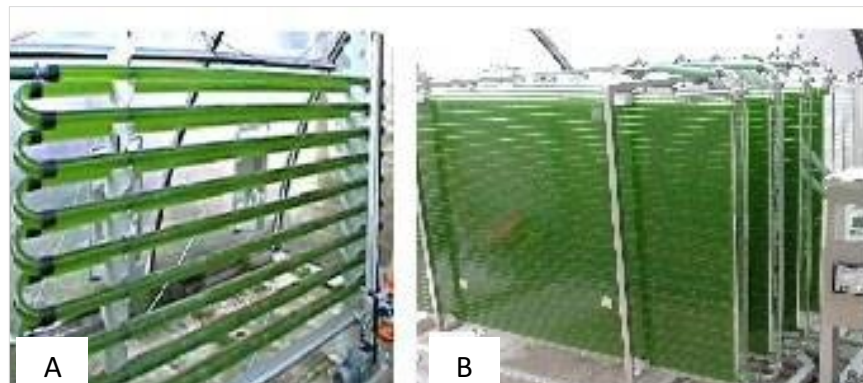
Figure 40. Different types of closed biospheres, A. Tubular photo-bioreactors, B. Flat sheet panel. Source: (Mata, Martins, & Caetano, 2010).
