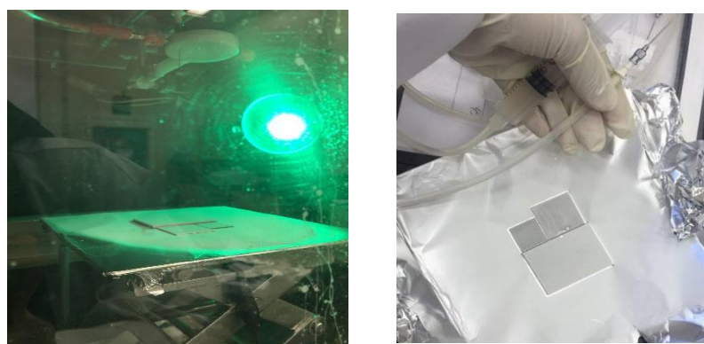
Figure 3.2. Coatings samples prepared via electrospinning technique
