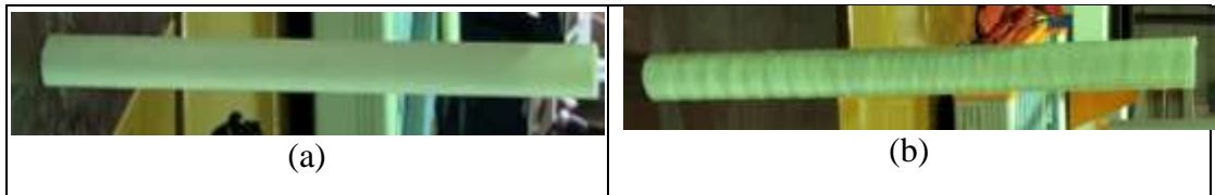
Figure 3.3 Prepared and fabricated specimens for examining the effect of the composite wrapping system on the bending behavior of plastic pipe (a) plastic pipe with 25 mm diameter (b) GFRP overwrapped plastic pipe with 25 mm diameter and fiber orientation of 55°.
