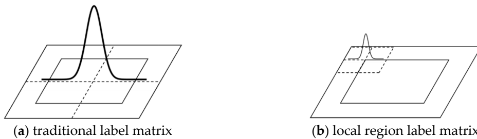
Figure 4. The comparison of label matrix between traditional circular samples and local region circular samples in time domain. The curves above the two label matrices denote the two-dimensional Gaussian distribution of both cases.
