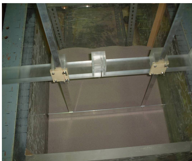
Figure 4: Manually-controlled instrument to form flat sand layers in the test container
