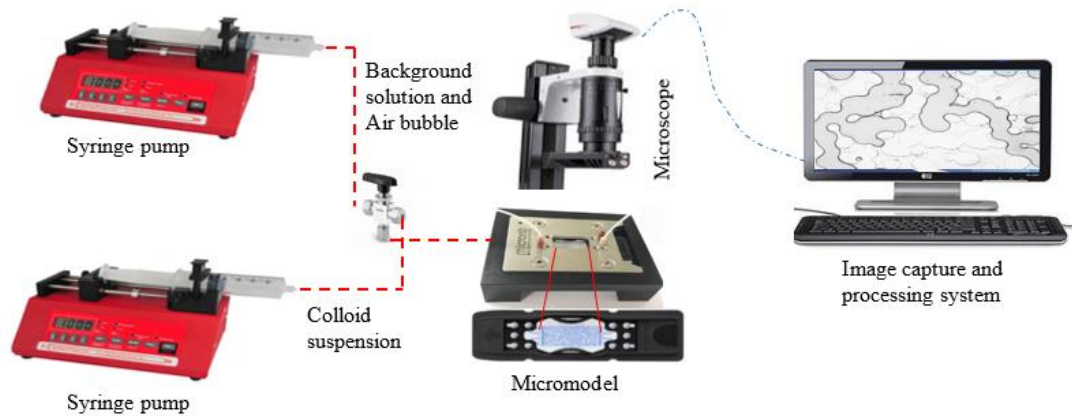
Figure 29. Experimental setup for the drainage and imbibition experiments in the micromodel. Drainage and imbibition were replicated by injecting trapped air bubbles and background solutions, respectively, to the micromodel.
