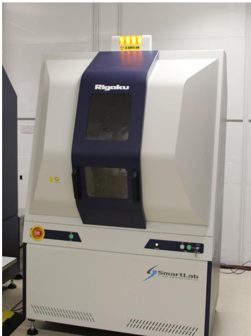
Figure 2-1: Rigaku X-ray diffraction combined with DSC unit (model: smart lab) (HBKU-QEERI-Core labs).
