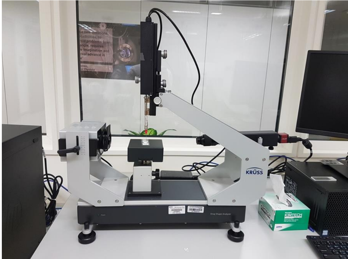
Figure 2-10: Kruss contact angle system. The sessile droplet method was used to calculate the contact angle for the samples in this study (HBKU-QEERI-Core labs).
