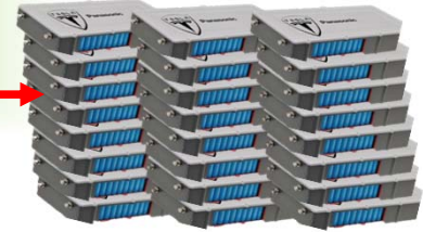
Higher number of battery cells are required to meet the 600V DC bus to drive the 3-phase IM drive
