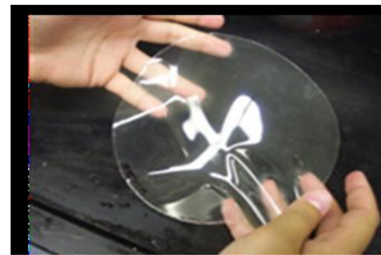
Figure 2: Sample for a polymeric membrane to be tested for carbon dioxide separation.
