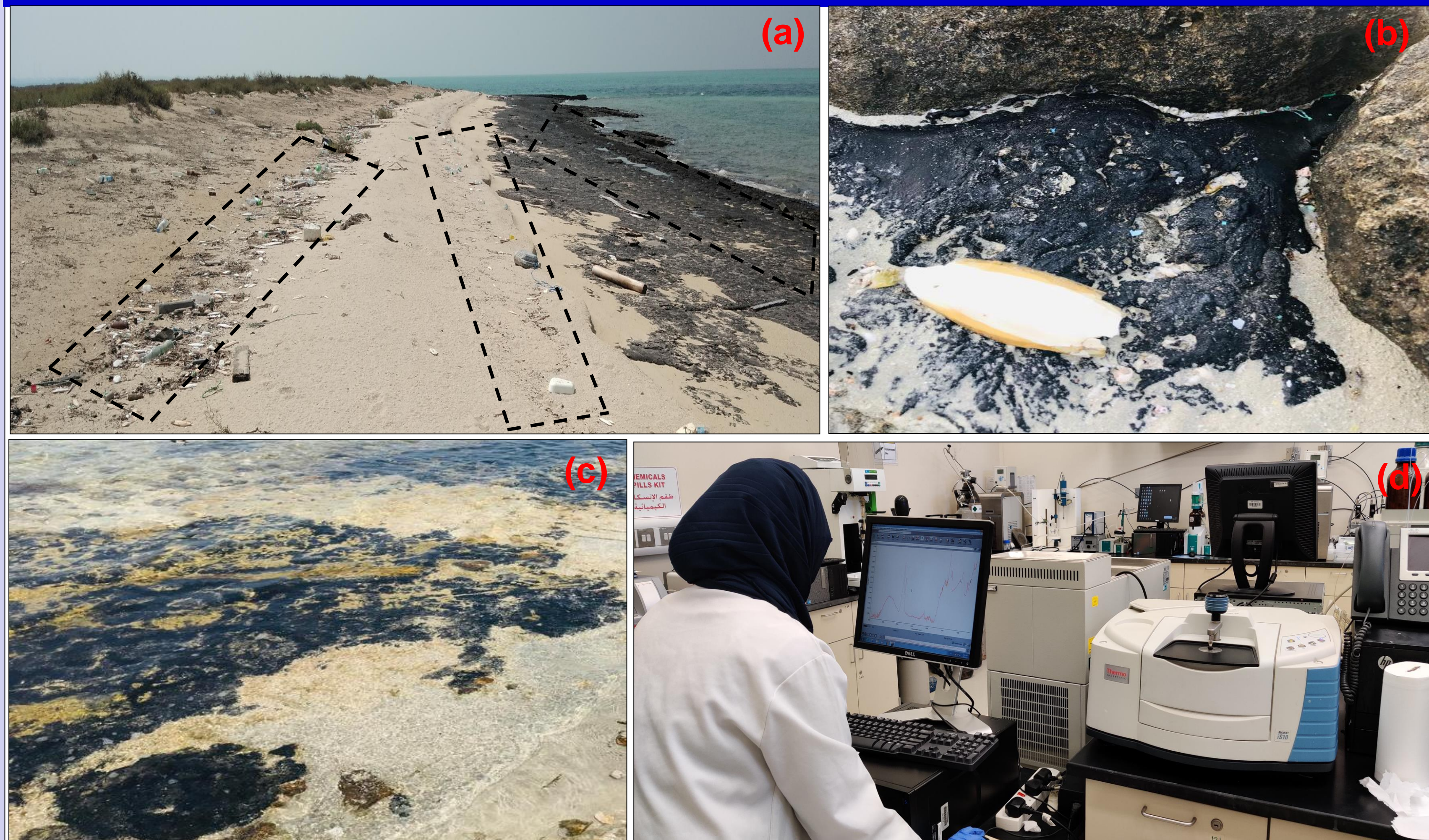
Figure 2 (a). Sampling transect in low tide, high tide and berm line; (b-c). Tarmats observed at Abu Samara and Al Zubara coasts, respectively and (d) ATR-FTIR analysis carried out at GPC, QU.
