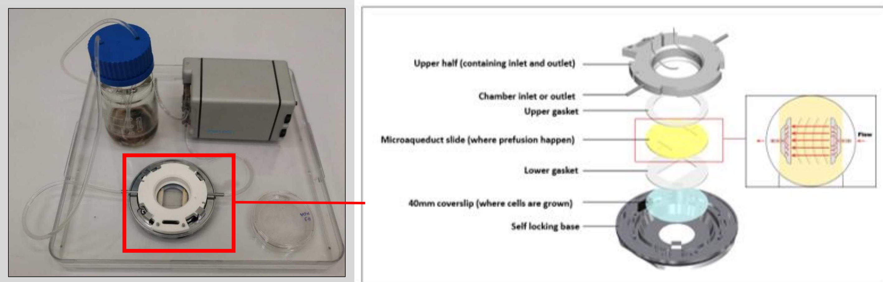
Figure 2: Breast cancer cells MDA-231 were grown in circular coverslips until confluence and assembled in a flow chamber. The flow chamber was connected to peristaltic pump at 0.1 dyn/cm 2 shear rate. The shear rate was calculated using Hagen-Poiseuille equation assuming a Newtonian fluid that has steady and laminar flow. MXene at 100ug/ml concentration was diluted in cell media and allowed to flow in the chamber to induce shear for four hours.
