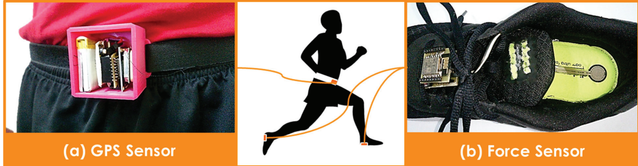
FIGURE 2. Sensor inputs used by microcontroller
