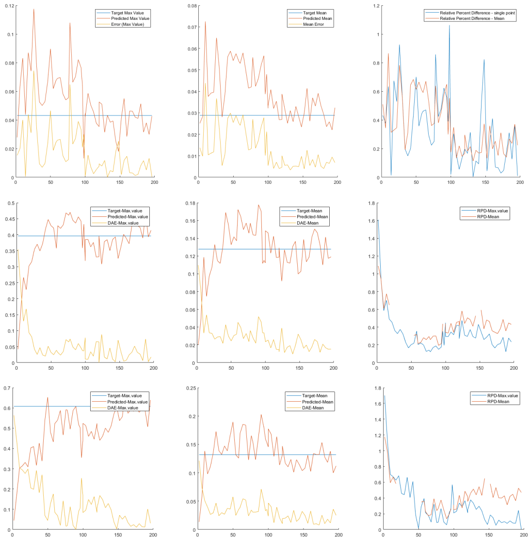
Figure 4.5: Force to Deflection model validation results of random samples across 200 Epochs
