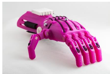
Figure 2. Anthropomorphic body-powered Raptor Reloaded prosthetic hand (© 2015 Walter Hsiao)
