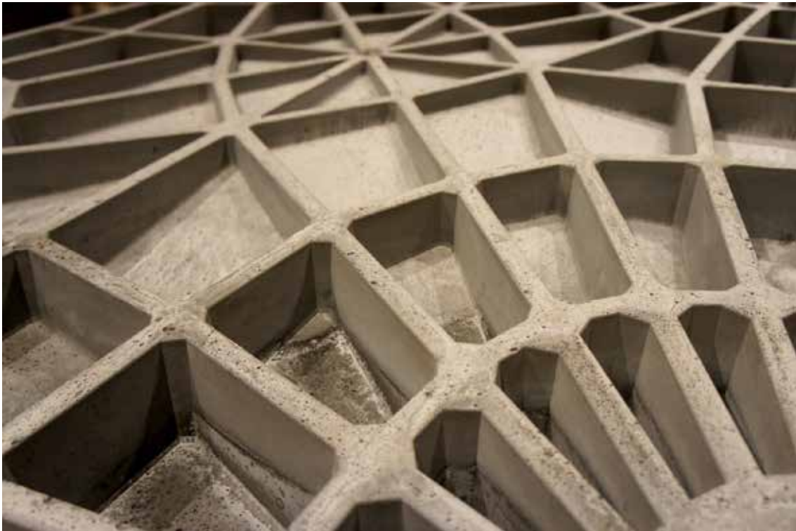
Figure 01: Mapungubwe Interpretive Centre, South Africa, 2008 and Rippmann Floor System prototype, 2016. The museum's tile vaults in soil-pressed tiles or the stiffened shell floor prototype are both thin, unreinforced structures using low-carbon-intensive material in very different contexts: soil-pressed tiles and concrete with a high percentage of recycled content. (Photos: Iwan Baan and Nick Krouwel)
