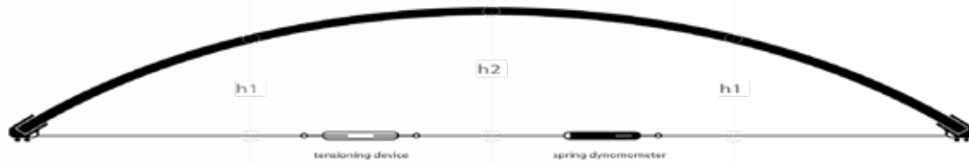
Figure 03: Bending physical test set-up.
