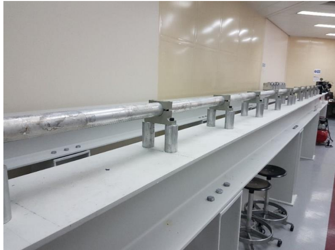
Figure 95. SHPB in structure laboratory
