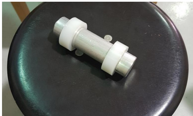
Figure 97. 150 mm Aluminum striker with UHMW Polyethylene rings
