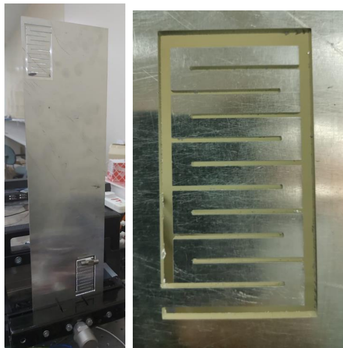
Figure 78. Experimental shaker setup of the Aluminum plate with cutout zigzag
