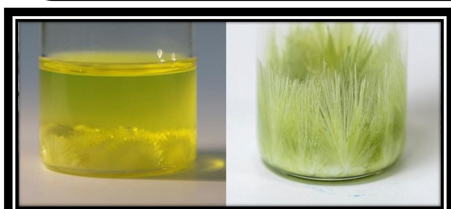
Figure 1: MAPbI 3 crystals grown in the DMF solution.
