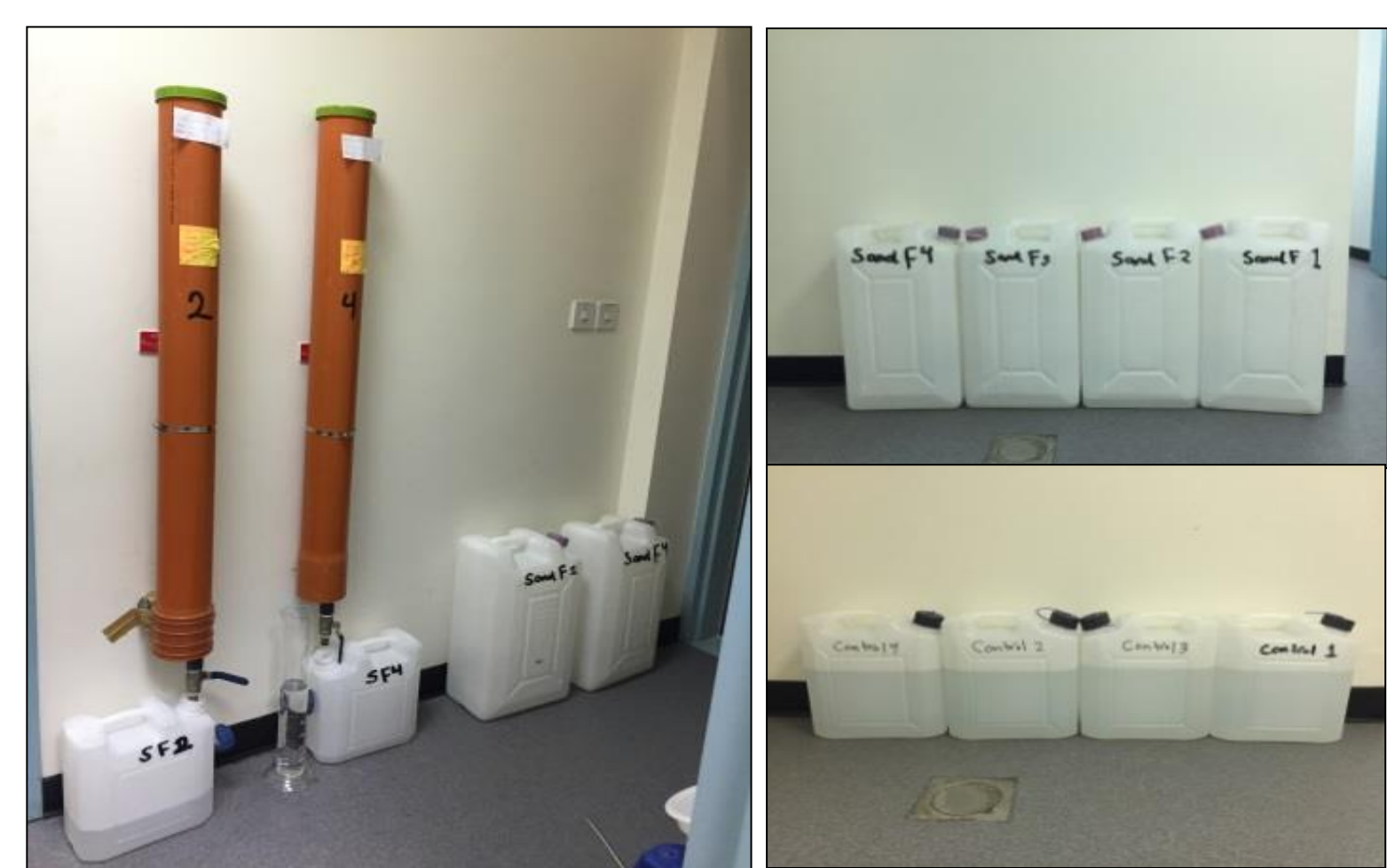
Figure 4: Sand filtration stage with Millipore water followed by produced water, collecting 4 controls samples and 4 samples.
