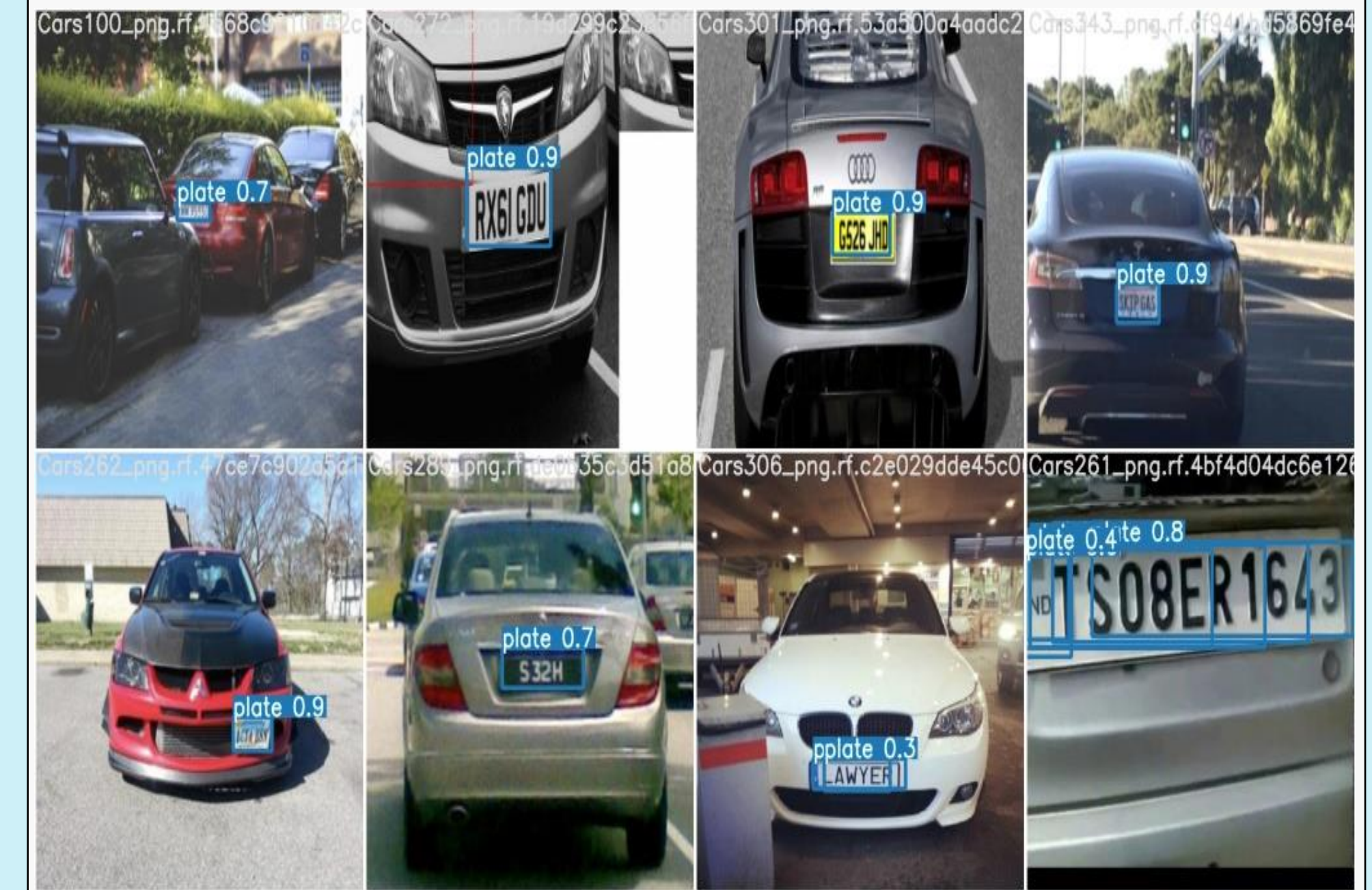
Figure 3, License plate detected test images with ground truth annotated
