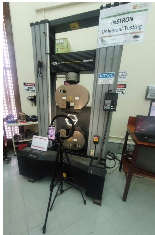
Figure 23: The setup of the compression testing.
