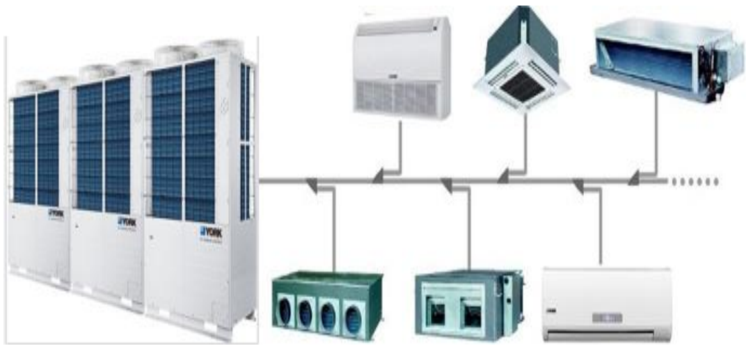
Figure 7 VRF system components [25]
