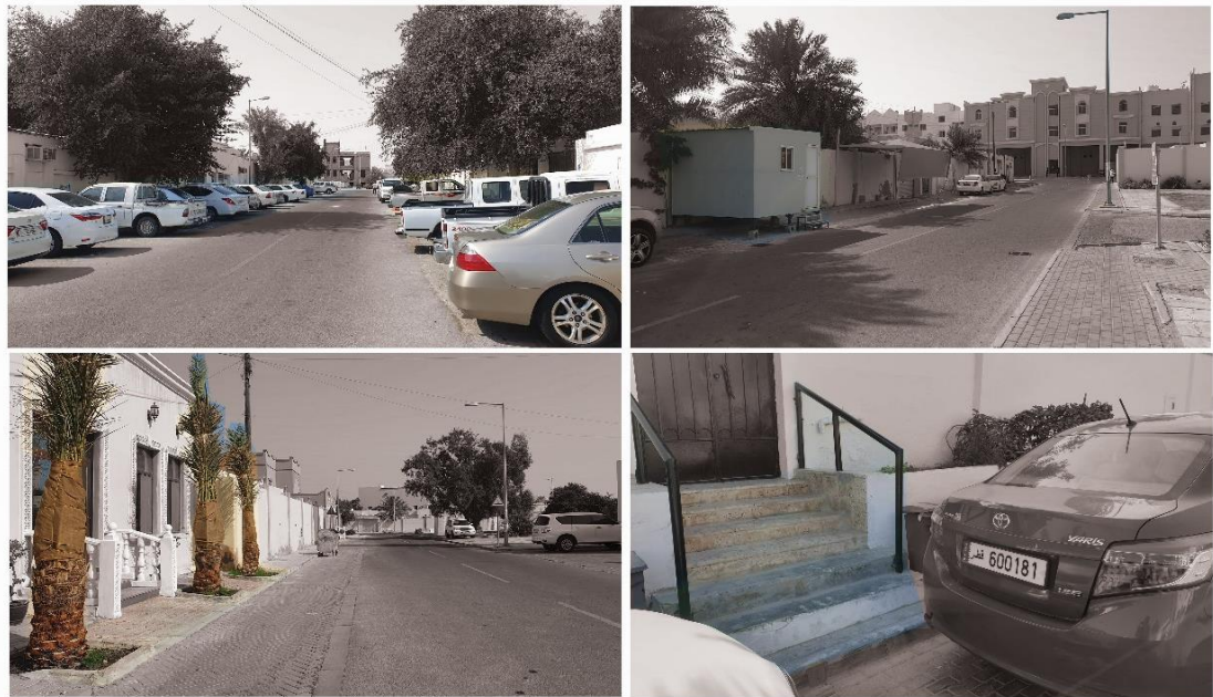
Figure 50. Some of the obstructions found along the sidewalk a) Cars parked along sidewalk on either sides b) Temporary mobile toilet along sidewalk c) Palm trees along sidewalk d) Steps jutting out in the sidewalk (clockwise from top left).
