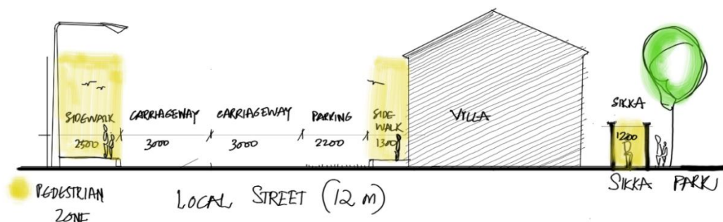
Figure 36. Typical section of sikkaks found in Madinat Khalifa south neighbourhood ranging from 1.2 m in width.
