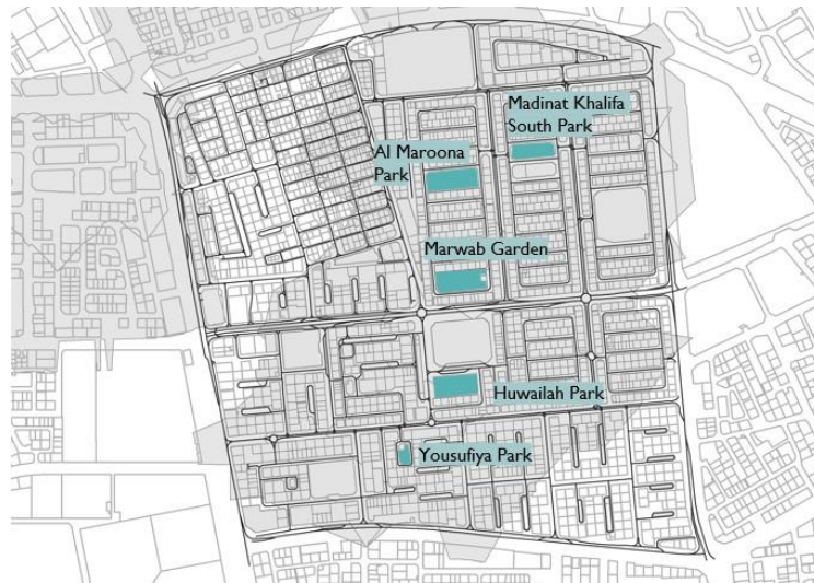
Figure 30. Area considered for Pedestrian Environment Data Scan (PEDS) walkability audit in Madinat Khalifa South neighbourhood within 5 minutes' walk around neighbourhood parks. Service area boundaries are obtained using network analysis tool in ArcMap within 400 m
